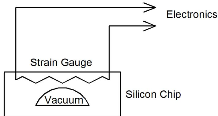
A strain gauge built into the chip is connected to the electronics to measure the pressure. All modern instruments are, of course, microcomputer based and schematically are a bit like this.
