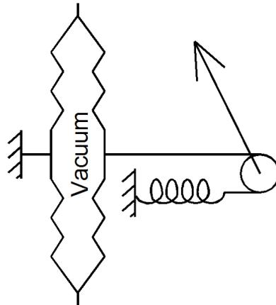
Mechanical altimeters work on this principle with a sort of diaphragm chamber called an aneroid which has a partial vacuum inside. As the altimeter goes up the reducing air pressure causes the chamber to expand and the needle to rotate.
