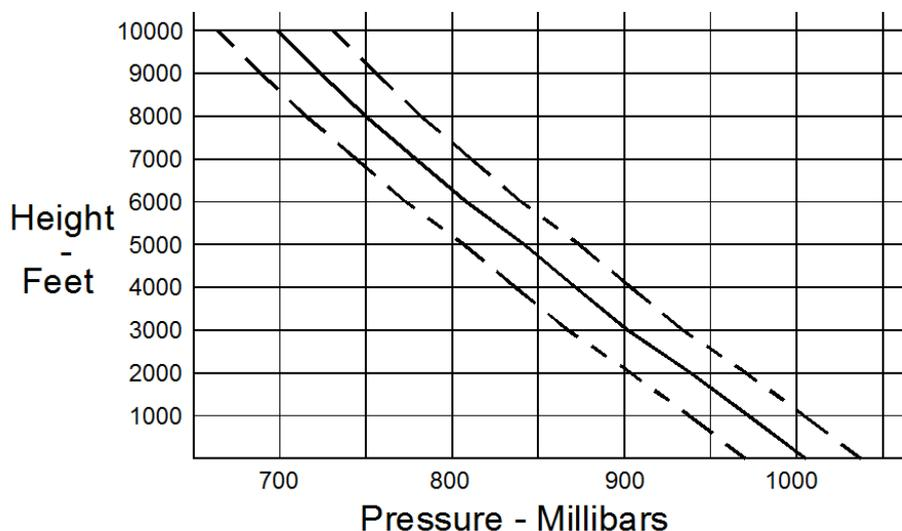
We have to adjust our altimeter to allow for these pressure changes. A standard aviation altimeter has a knob for doing this.
