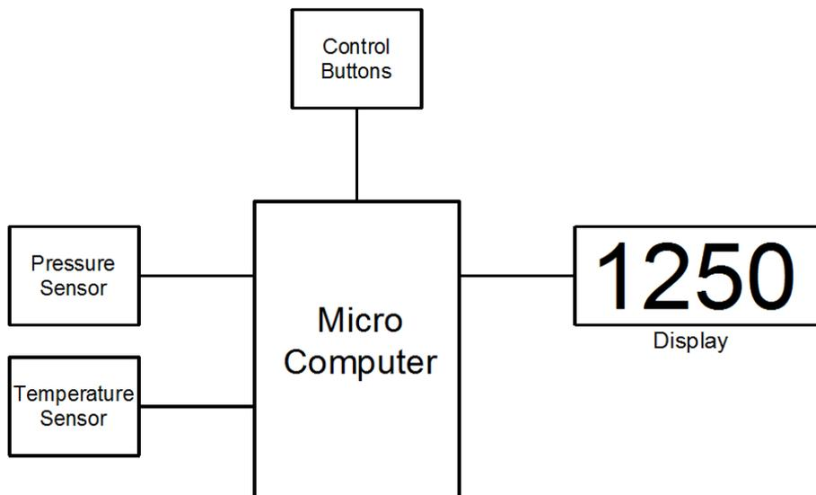
Information from the pressure sensor is interpreted by the microcomputer and sent to the display. Because pressure sensors are also sensitive to temperature we also have a temperature sensor so the microcomputer can apply compensation for temperature changes.
